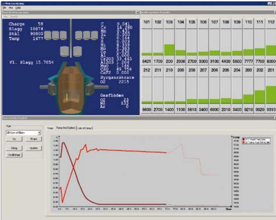
Figure 6 - Tracking and prediction view
