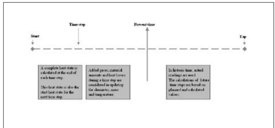
Figure 6 – Tracking and prediction principle
