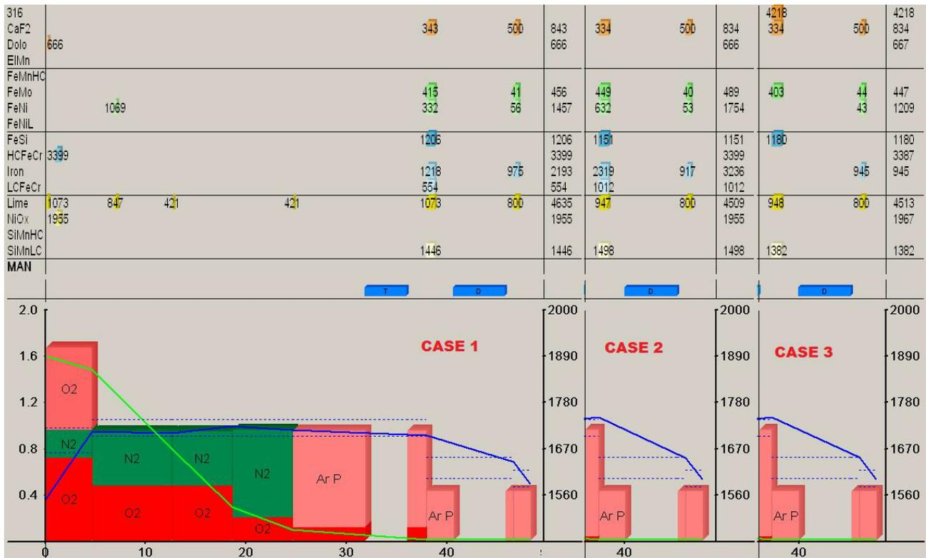
Fig. 3: A scenario predicted prior to a high temperature measurement (case 1) and as re-calculated after the high temperature measurement when granulated AISI 316 is available (case 3) and when cooling with alloys is used (case 2)
