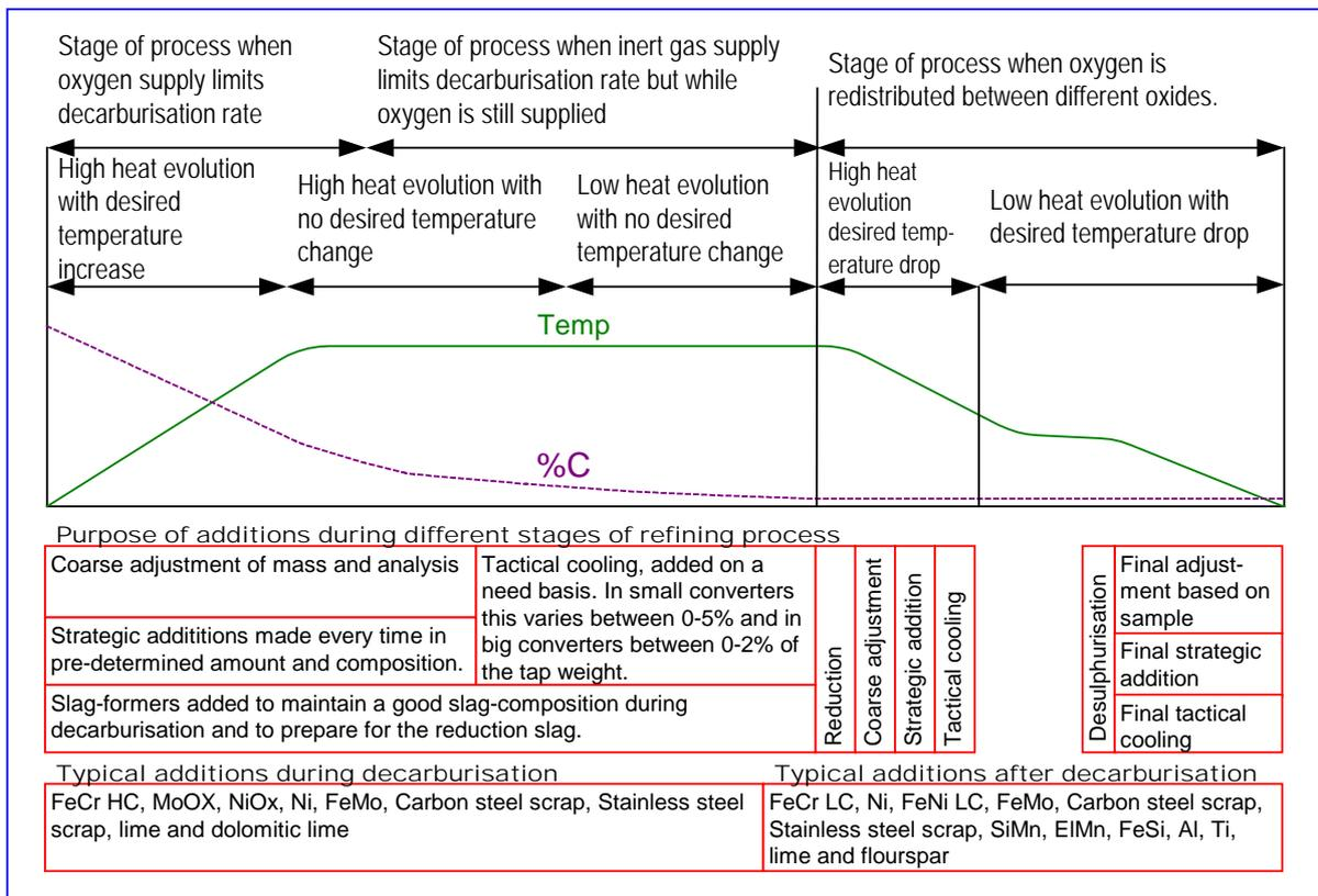
Fig. 1: Typical cold material distribution and purposes during AOD refining
