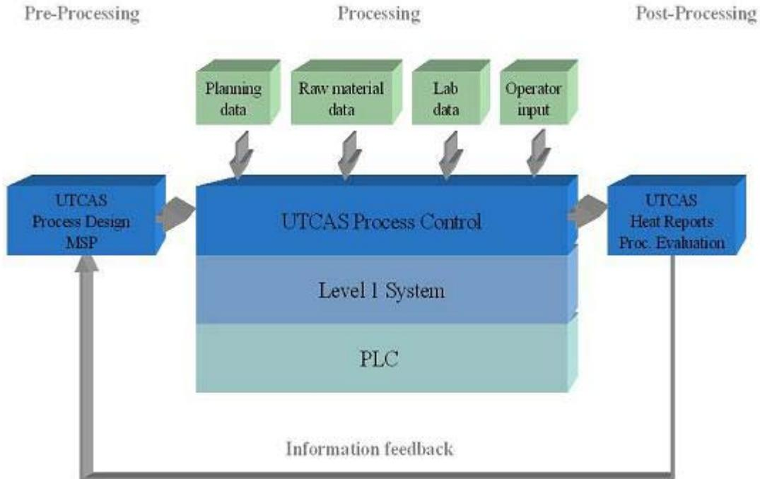
Fig. 2: The UTCAS concept for process control and management.
