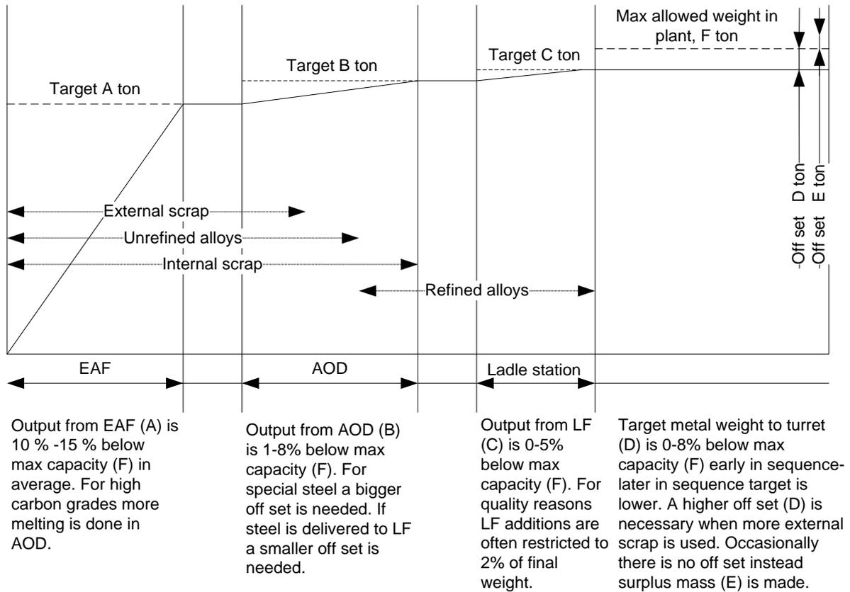
Figure 1. Mass build-up throughout the melt shop.
