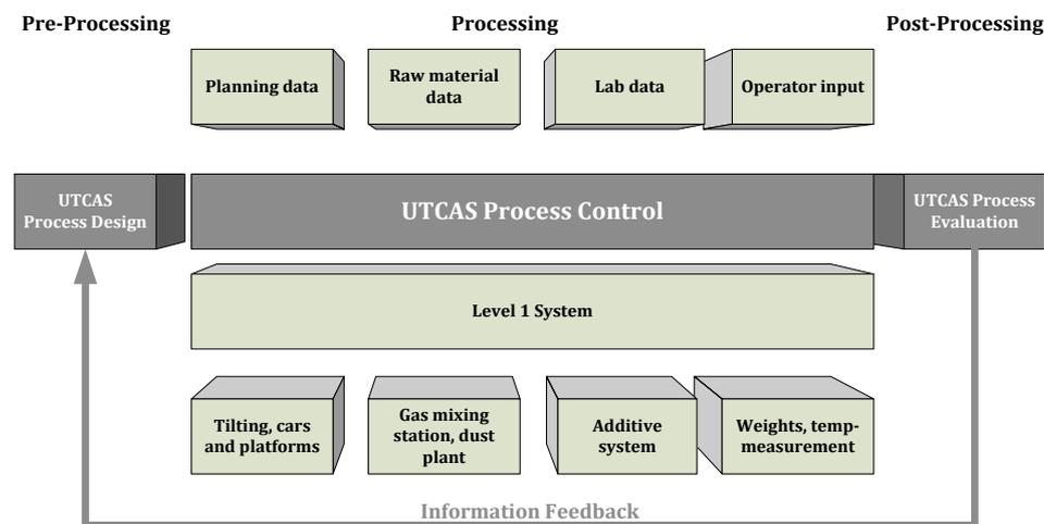
Figure 3. The UTCAS® concept for process control and management.
