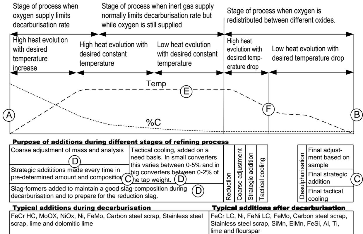
Figure 2. Alloy and scrap additions during the AOD process.
