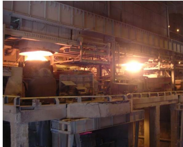
Figure 2. Columbus twin 120 t converters are operating with steam as a process gas.
