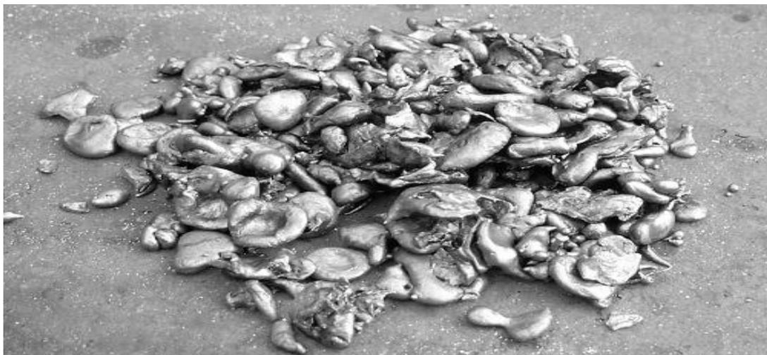
Figure 4 Granulated Pig Iron (GPI™) produced at Saldanha Steel
