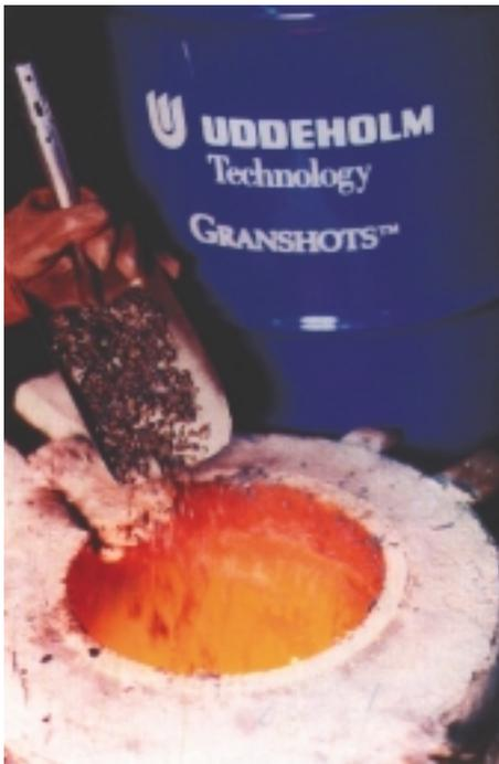
Fig 2. Charging GRANSHOT into a furnace
