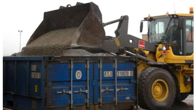
Fig 4. Granulated recycled stainless steel dust being packed.
