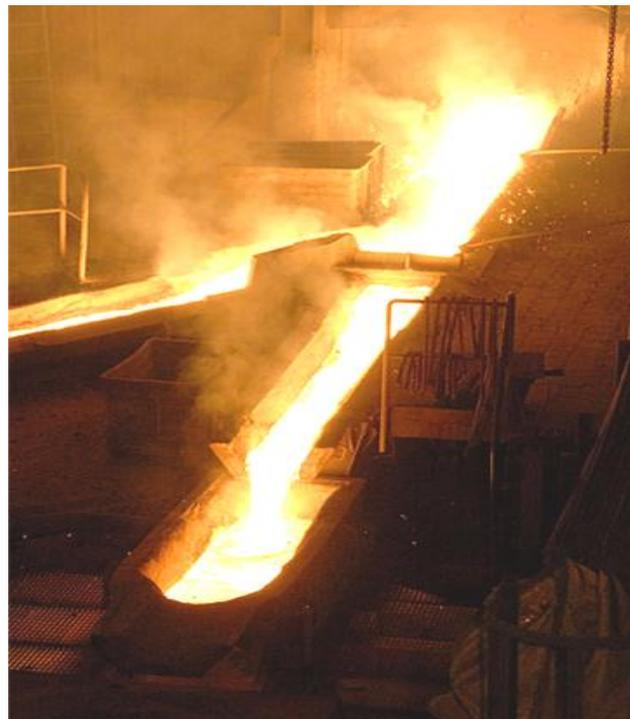
Fig 2. Hot liquid metal directly enters the granulation tundish.
