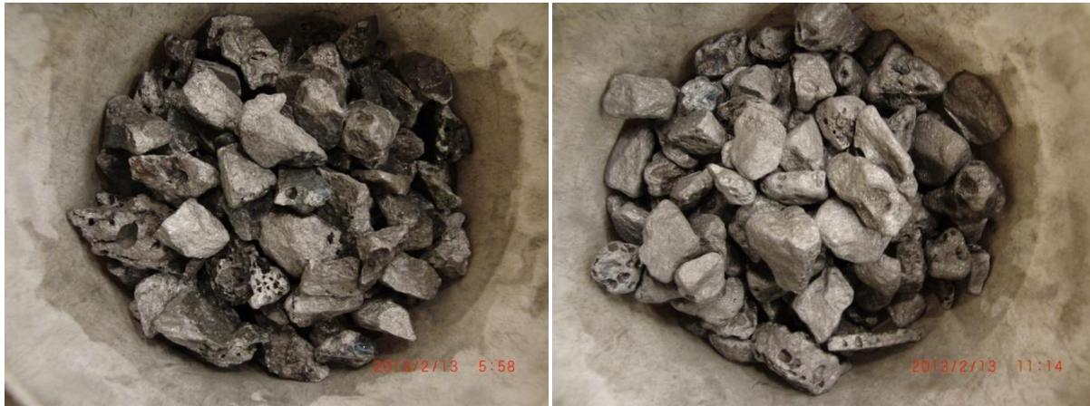
Figure 9. Crushed HC FeCr before (left) and after 30 min tumbling (right).
