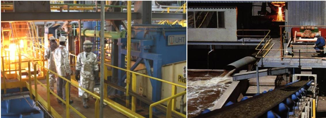
*Figure 3. FeNi granulation at VALE Onca Puma, Brazil (left) and granulation of FeCr at SAMANCOR Ferrometals, South Africa (right).*
