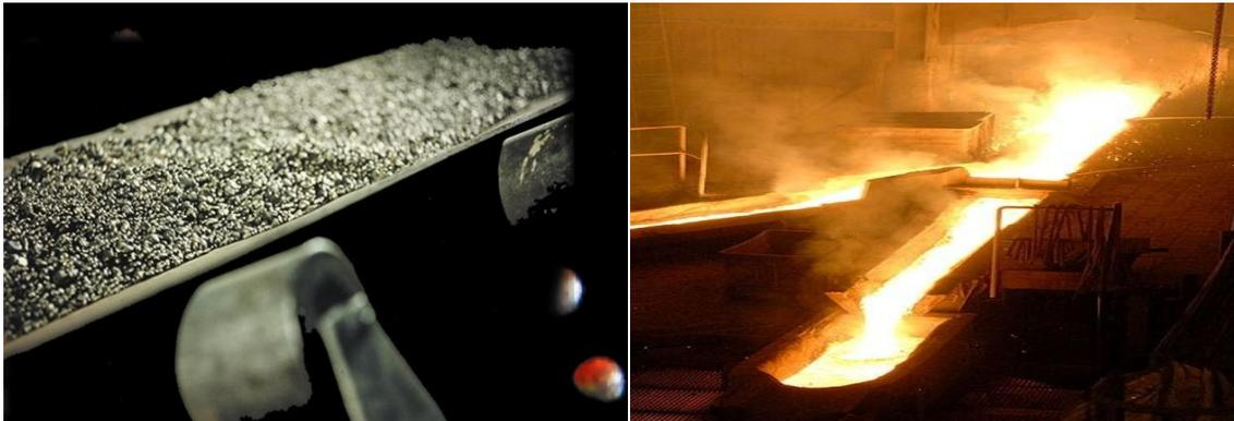
*Figure 12. Granulated ferroalloy can be handled by conveyors and silos (left). Tapping directly from the furnace to the GRANSHOT unit saves on operational cost (right).*
