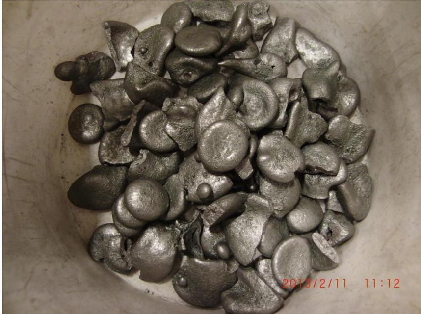
*Figure 11. Granulated 16-25 mm HC FeCr after 30 min tumbling. Still the same shape of granule with some broken into two pieces.*
