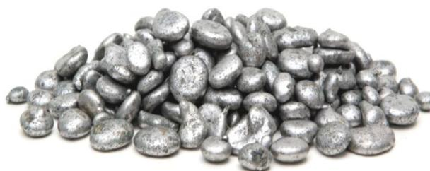
*Figure 2. Hot metal hits the refractory sprayhead, producing droplets (left), cooled in water tank below as to make solid granules, here FeCr (right).*
