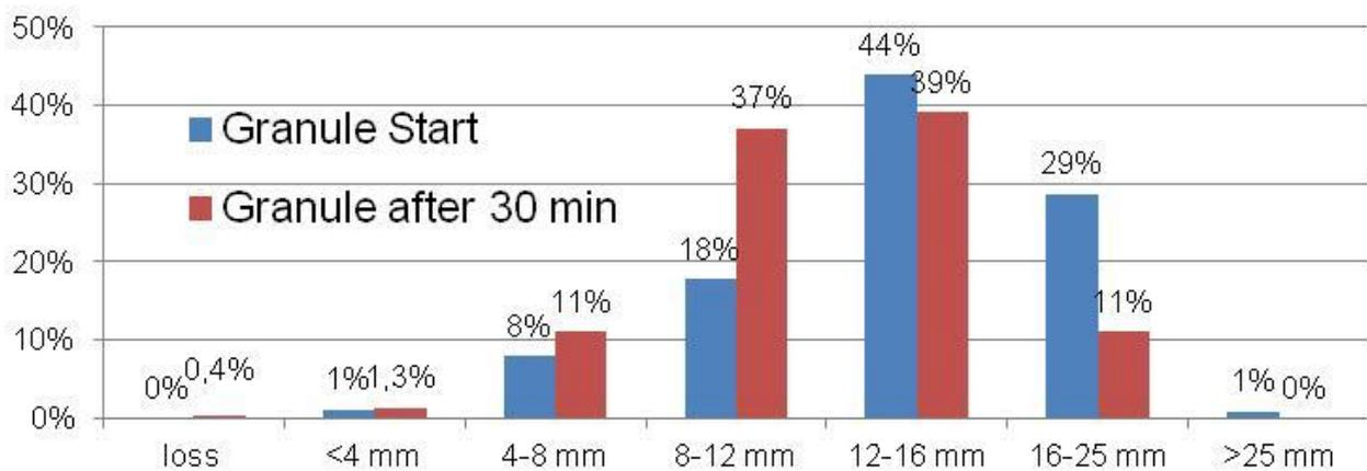
Figure 7. Percentage (%) of size fractions of Granulated HC FeCr, before (Start) and after 30 min of tumbling.
