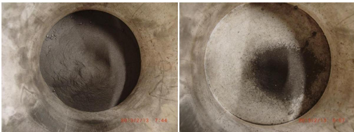
Figure 10. After 30 min of tumbling, fines of crushed (left) and for granulated HC FeCr (right)
