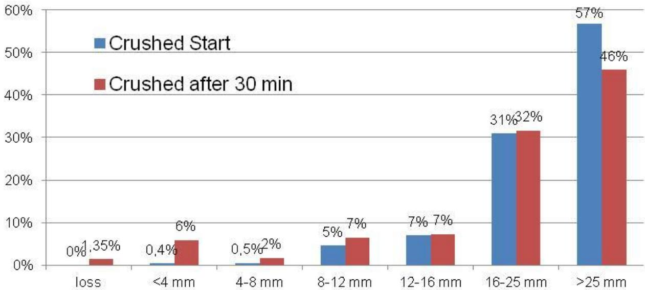
Figure 6. Percentage (%) of size fractions of Crushed HC FeCr, before (Start) and after 30 minutes after tumbling.
