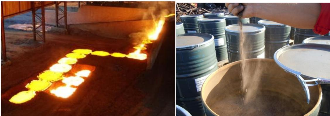
*Figure 1. Dry-pit or pan casting (left) & crushing of ferroalloys results in high levels of fines. Dust-like FeCr 0-10 mm fines (right) has limited value in steel making.*
