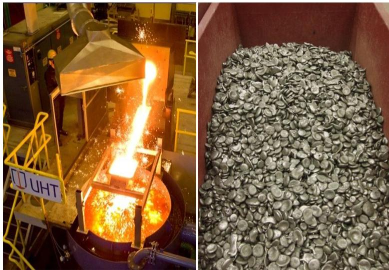
*Figure 5. HC FeCr melted in Pilot granulation unit (left) to produce FeCr granules (right).*
